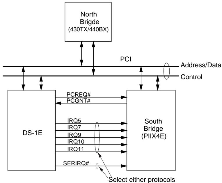
The PCI-to-ISA bridge needs to support PC/PCI. IRQ is directly connected to the IRQ input pins on the PCI-to-ISA bridge.
