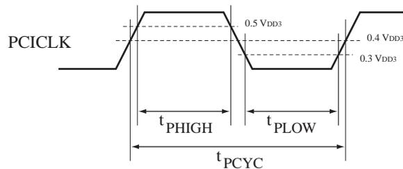
Fig.3: PCI Clock timing
