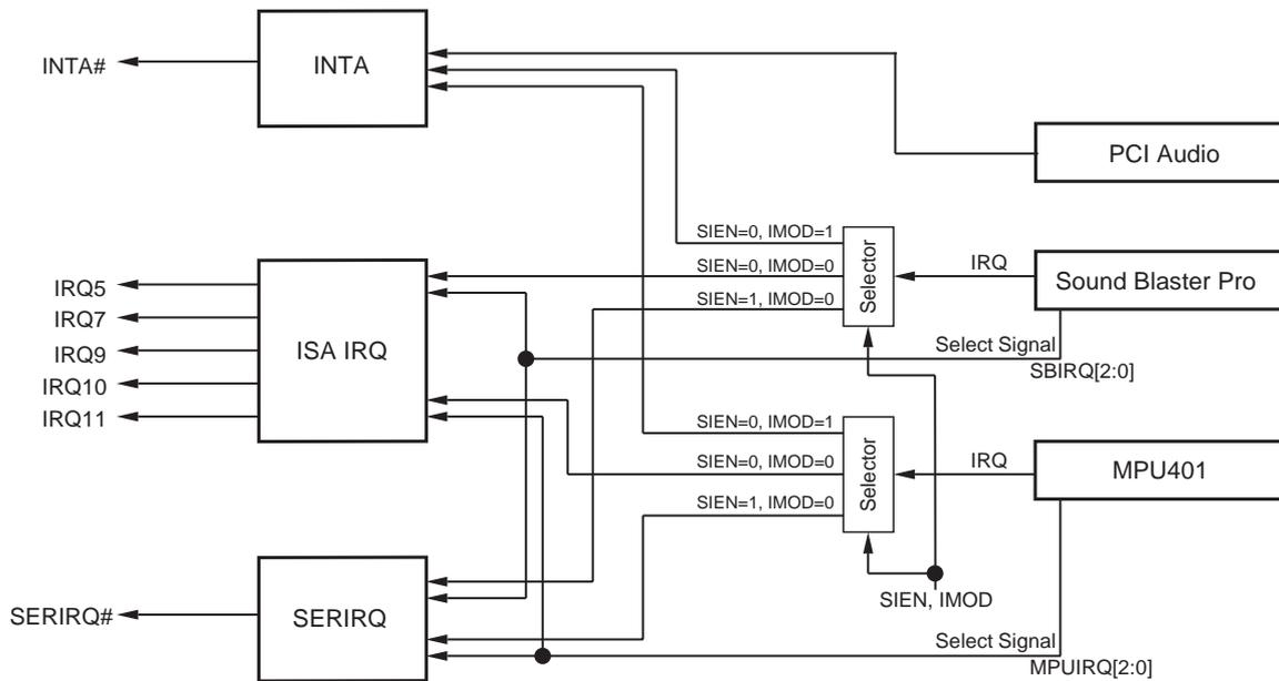
PCI Audio can only use INTA#, but the Sound Blaster Pro and MPU401 blocks of the Legacy Audio Block can use any of the three protocols.
