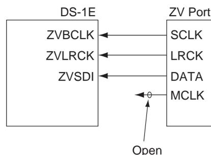
The Zoomed Video Port is used to be selected between SPDIF input on YMF744B (DS-1S). However, on DS-1E, the both functions can be used at the same time.
