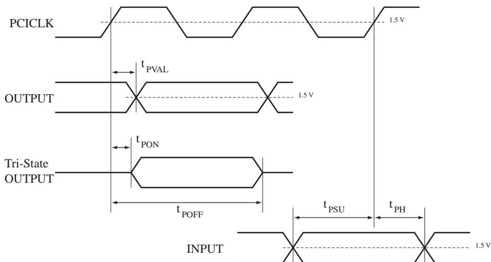
Fig.4: PCI Bus Signals timing
