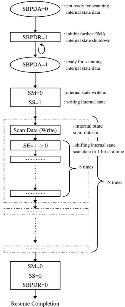
$$N = 34 \text{ byte (Total Scan Data = 268 bit (33 byte} \times 8 + 4 \text{ bit))}$$
