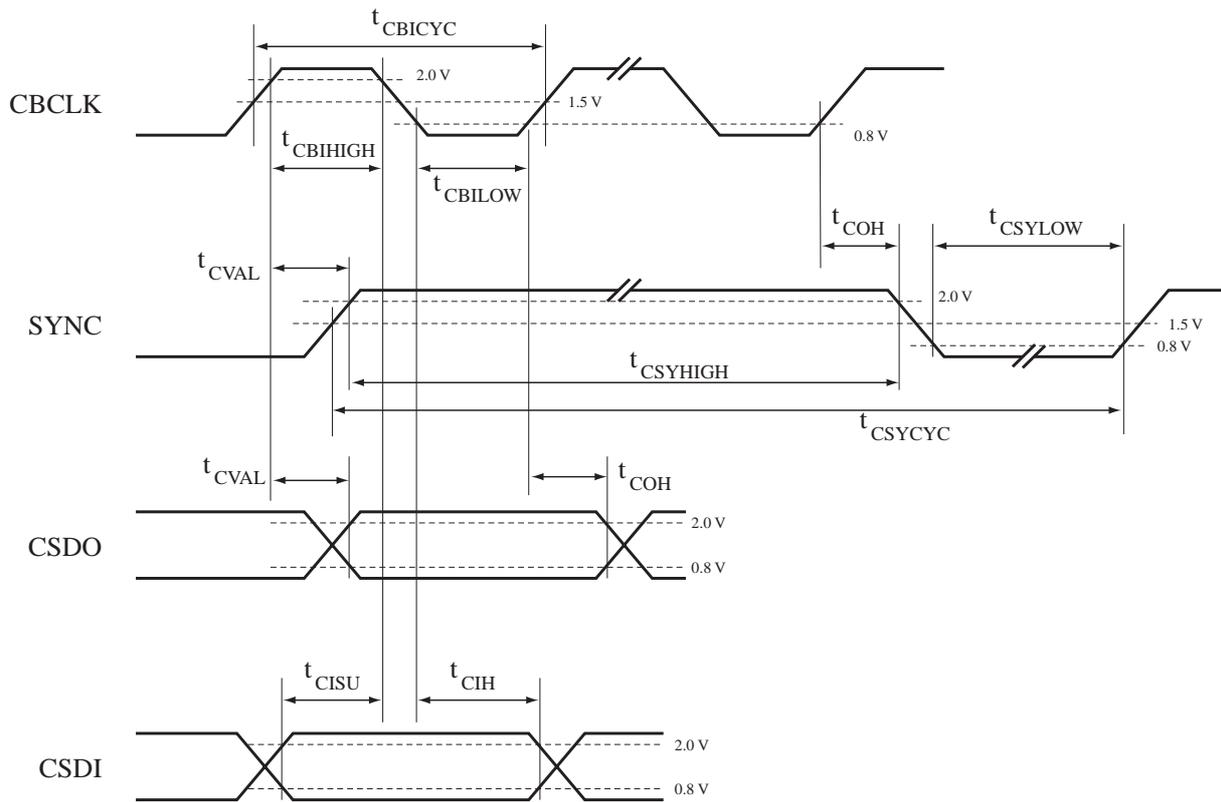
Fig.6: AC-link timing
