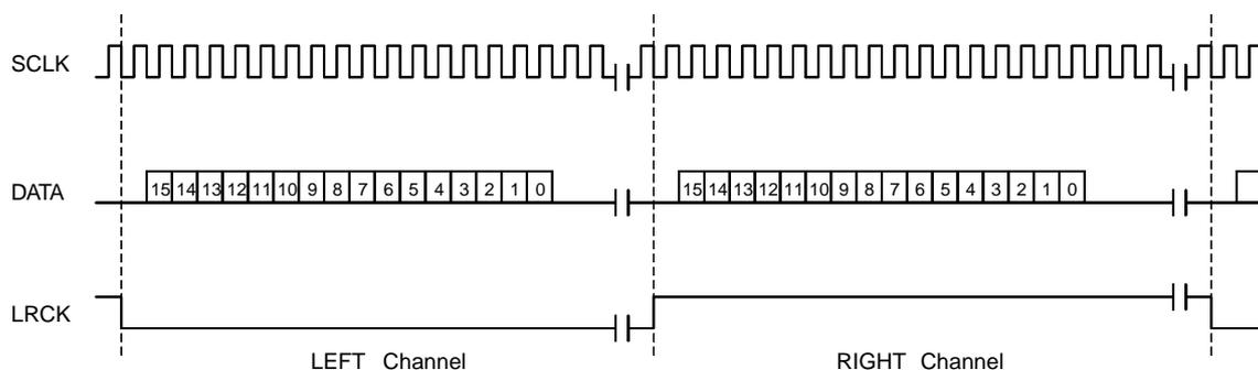
In the Zoomed Video Port, synchronization with a master clock supplied from the bus is inherently required. However, DS-1E can asynchronously process audio signal input via the Zoomed Video Port, eliminating the need for master clock.
