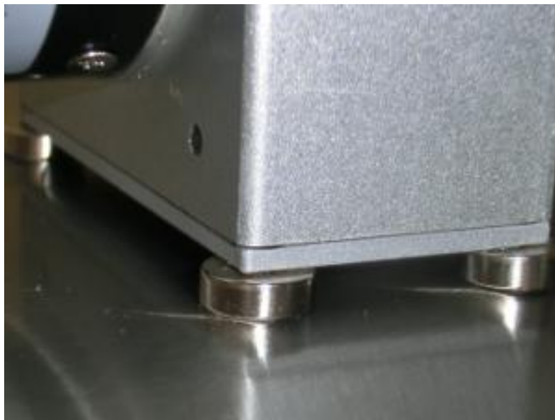
Figure 7.1: Magnets on a metal surface
