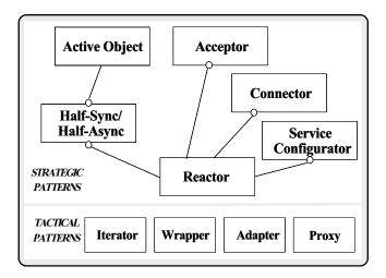
The Event Channel components are based upon a system of design patterns
