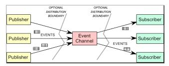
Figure 1: Relationships Between Components in a Publisher/Subscriber Architecture
