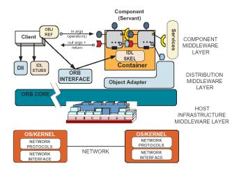
Figure 2: Layered CCM Architecture
