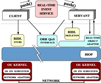
Figure 4: Architecture of the TAO ORB Endsystem
