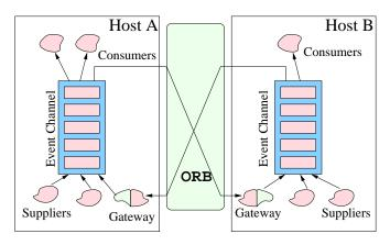
Figure 8: A Federated Event Channel Configuration
