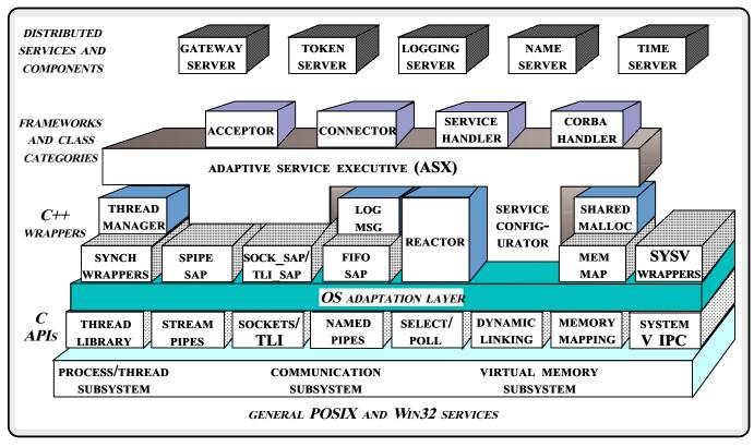
Figure 1: Components in the ADAPTIVE Communication Environment
