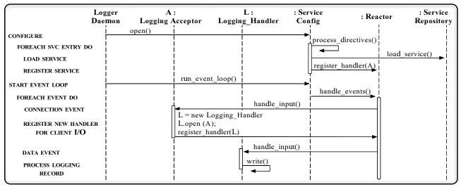
Figure 16: Interaction Diagram for the Server Logging Daemon
