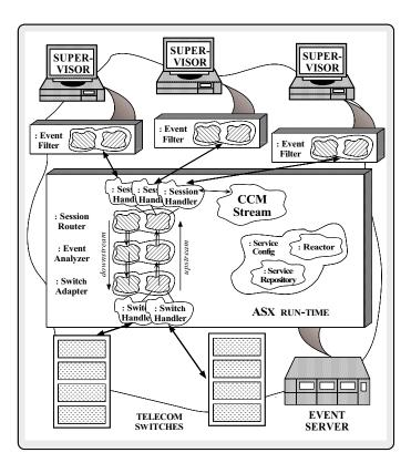
Figure 18: Reconfiguration of PBX Monitoring System
