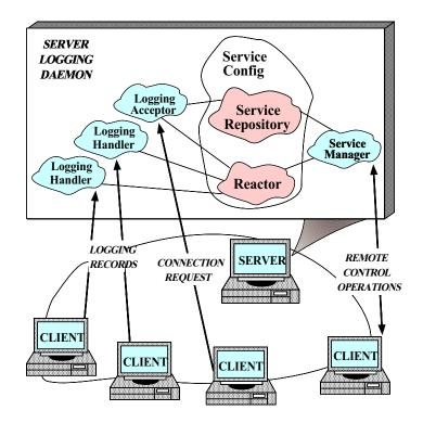
Figure 15: ACE Components in the Distributed Logging Facility
