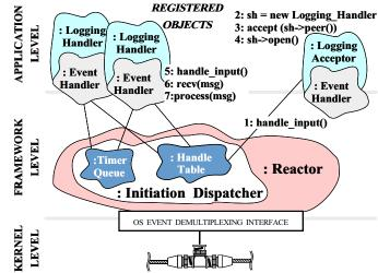
Figure 6: The ACE\_Reactor Class Category Components
