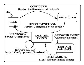
Figure 10: State Transition Diagram for Service Configuration, Execution, and Reconfiguration
