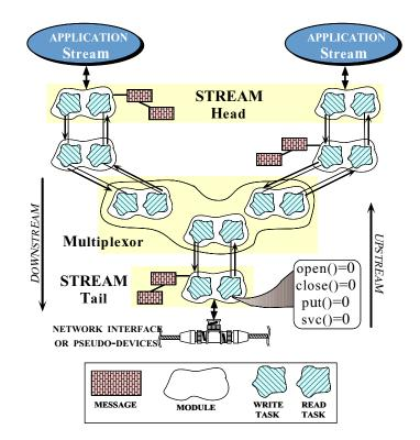
Figure 11: Components in the ASX Framework
