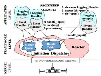
Figure 5: Software Architecture of the WWW Server
