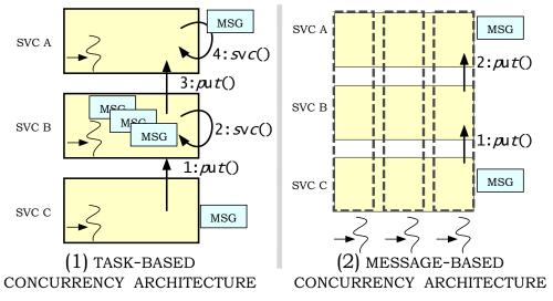
Figure 12: Alternative Methods for Invoking put and svc Methods
