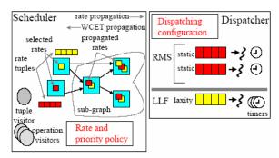
Figure 5: Reconfigurable Scheduler and Event Channel Dispatcher Interoperation in TAO
