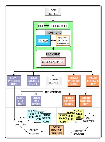
Figure 4: Design and Use of the DCE $\rightarrow$ CORBA Migration Tool
