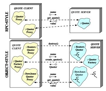
Figure 2: RPC-style vs. Object-style Communication
