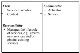
Our example uses thread-based service execution contexts to run automation services implemented as C++ objects. After activating a service, the service execution context invokes a method on the service to initialize itself.
