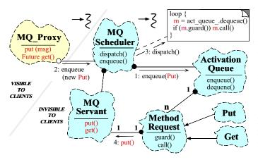
Figure 2: Implementing a Message Queue as an Active Object for Consumer Handlers
