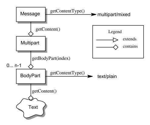
In this figure, the ContentType attribute of a Message object indicates that it holds a multipart content. Use the getContent() method to obtain the Multipart object.
