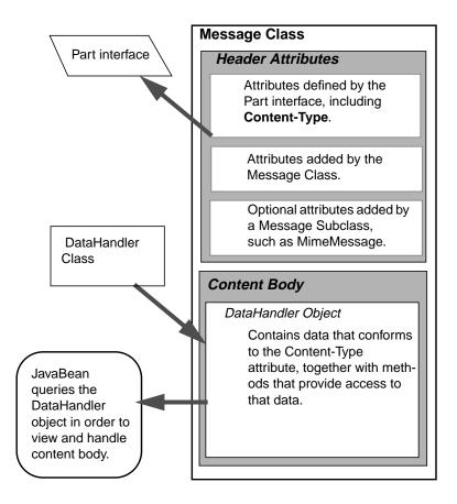
The Message object has no direct knowledge of the nature or semantics of its content. This separation of structure from content allows the message object to contain any arbitrary content.
