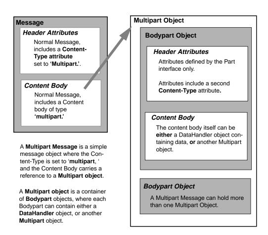
Note that Multipart objects can be nested to any reasonable depth within a Multipart Message, in order to build an appropriate structure for data carried in DataHandler objects. Therefore, it is important to check the ContentType header for each BodyPart element stored within a Multipart container. The figure below illustrates a typical nested Multipart Message.
