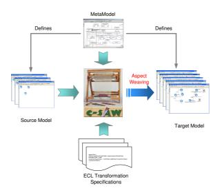
Fig. 7. C-SAW Aspect Model Weaver Framework
