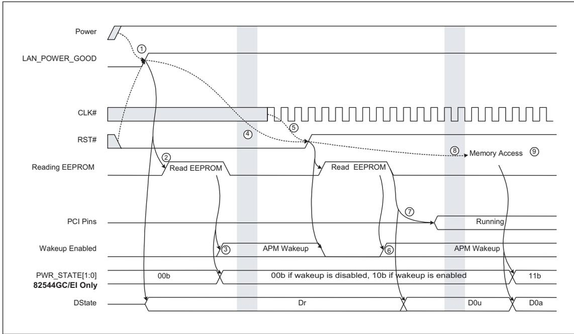
Figure 6-2. Startup Timing
