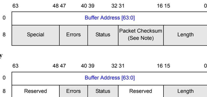
**Note:** The checksum indicated here is the unadjusted “16 bit ones complement” of the packet. A software assist may be required to back out appropriate information prior to sending it to upper software
