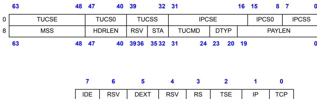
**Figure 3-6. TCP/IP Context Transmit Descriptor & Command Layout**
