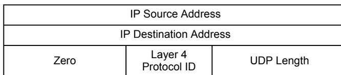
Figure 3-17. UDP Pseudo Header Diagram for IPv4
