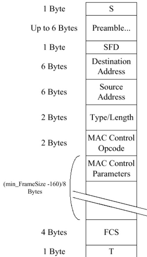
**Note:** “S” is the Start-of-Packet delimiter and “T” is the first part of the End-of-Packet delimiters for 802.3z encapsulation.
