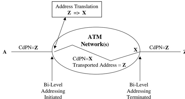
**Figure 3-1 ATM Bi-Level Addressing Concept**
