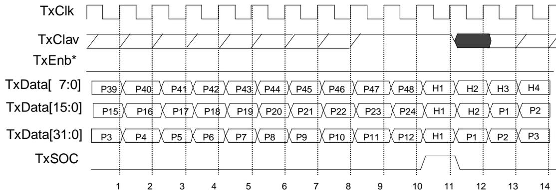
**Figure 3.1: Transmission of two cells back-to-back**
