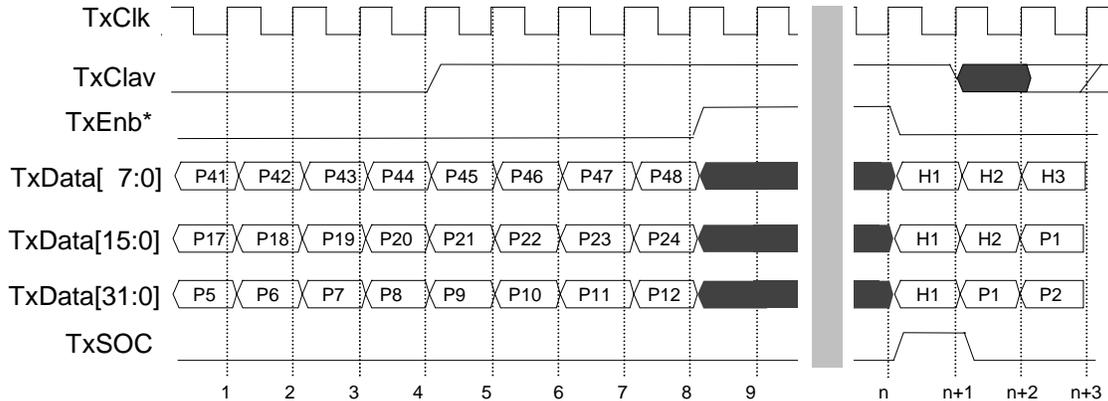
**Figure 3.2: Transmission stalled by the ATM layer device**
