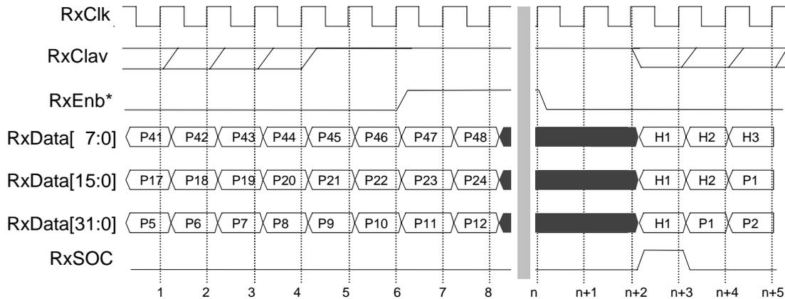
**Figure 3.5: Reception stalled by the ATM layer device**
