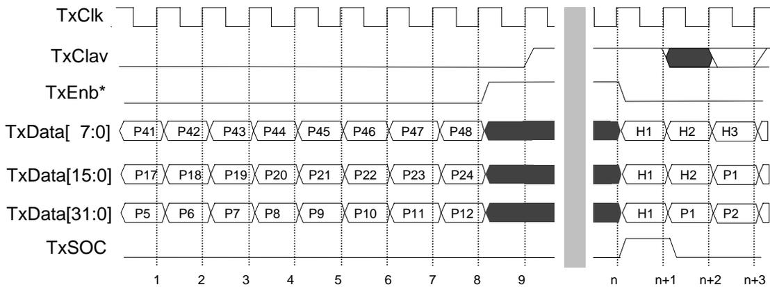
**Figure 3.3: PHY layer device not ready to receive cell**
