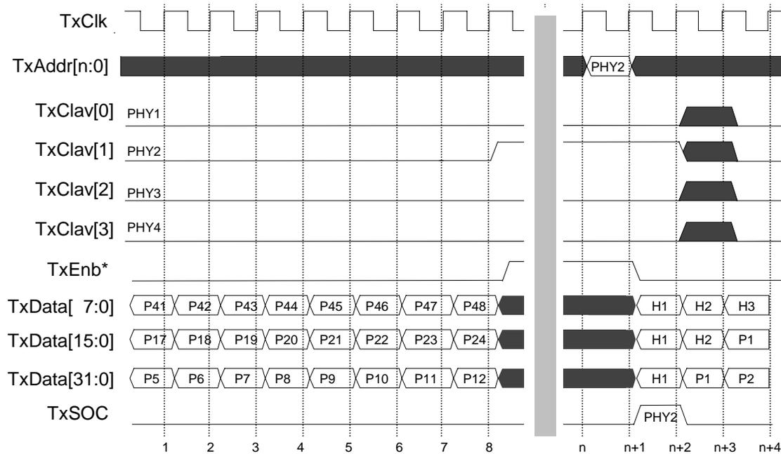
**Figure 4.3: PHY layer device not ready to receive cell**
