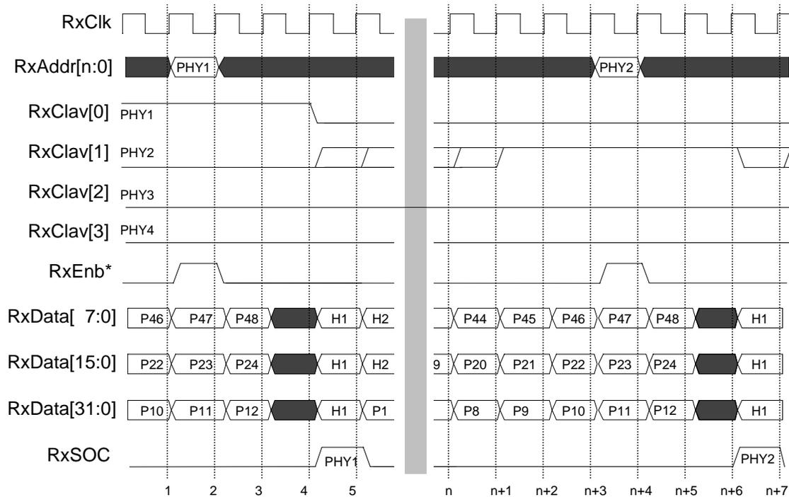
**Figure 4.4: Receive Decode and Selection**
