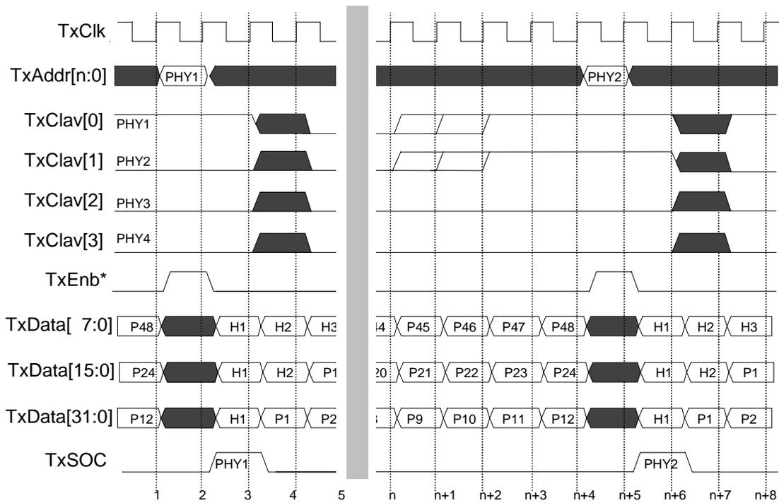
Figure 4.1: Transmit Decode and Selection
