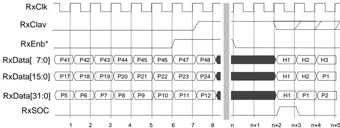
**Figure 3.6: PHY layer device not ready to transmit cell**
