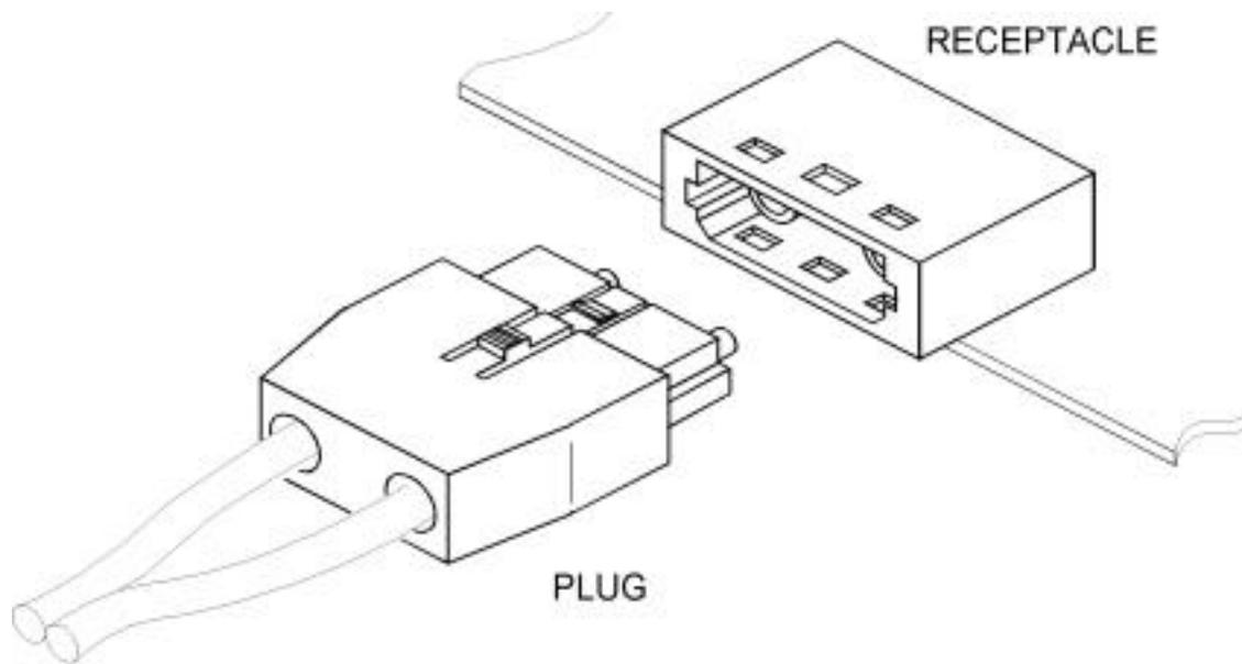
**Figure 1a Physical Media Plug and Receptacle
