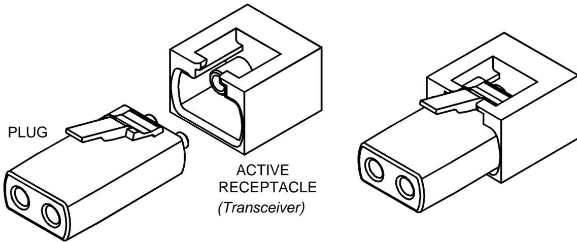
**Figure 1b Physical Media Plug and Receptacle
