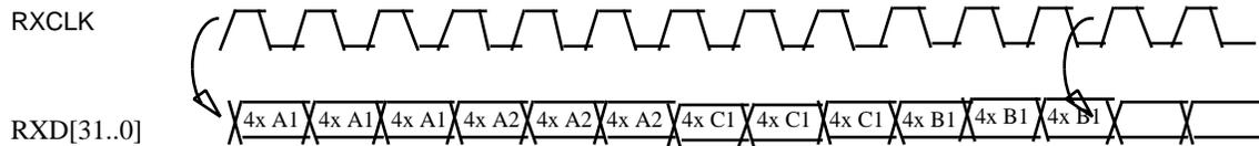
**Figure 13: 32 Bit Receive Side Timing From PMD To TC**
