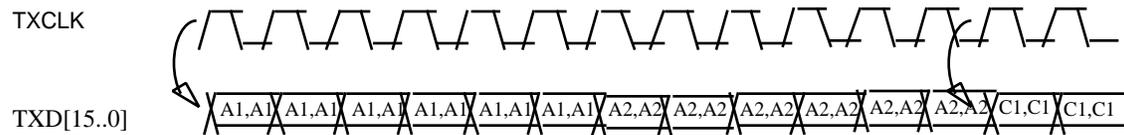
**Figure 8: 16 Bit Transmit Side Timing From TC To PMD**
