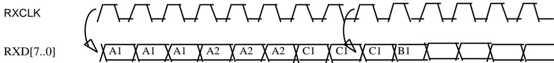
**Figure 7: 8 Bit Receive Side Timing From PMD To TC**
