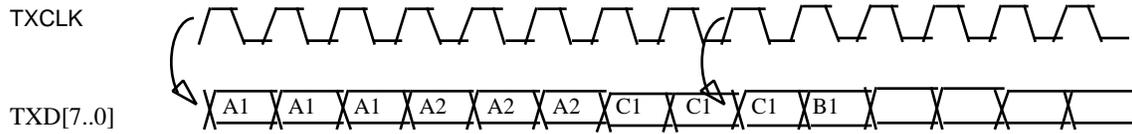
**Figure 6: 8 Bit Transmit Side Timing From TC To PMD**
