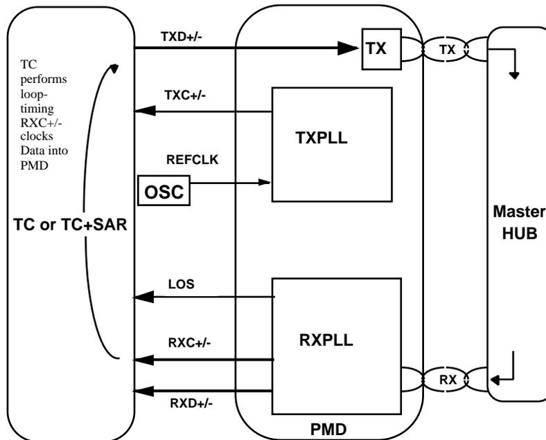
**Figure 16: Serial Interface Setup End Unit (Clock Slave)**
