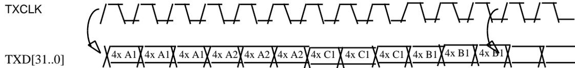
**Figure 12: 32 Bit Transmit Side Timing From TC To PMD**
