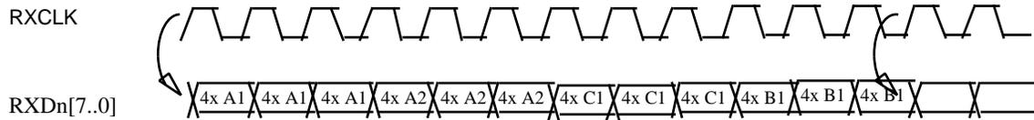
**Figure 11: Quad 8 Bit Receive Side Timing From PMD To TC**
