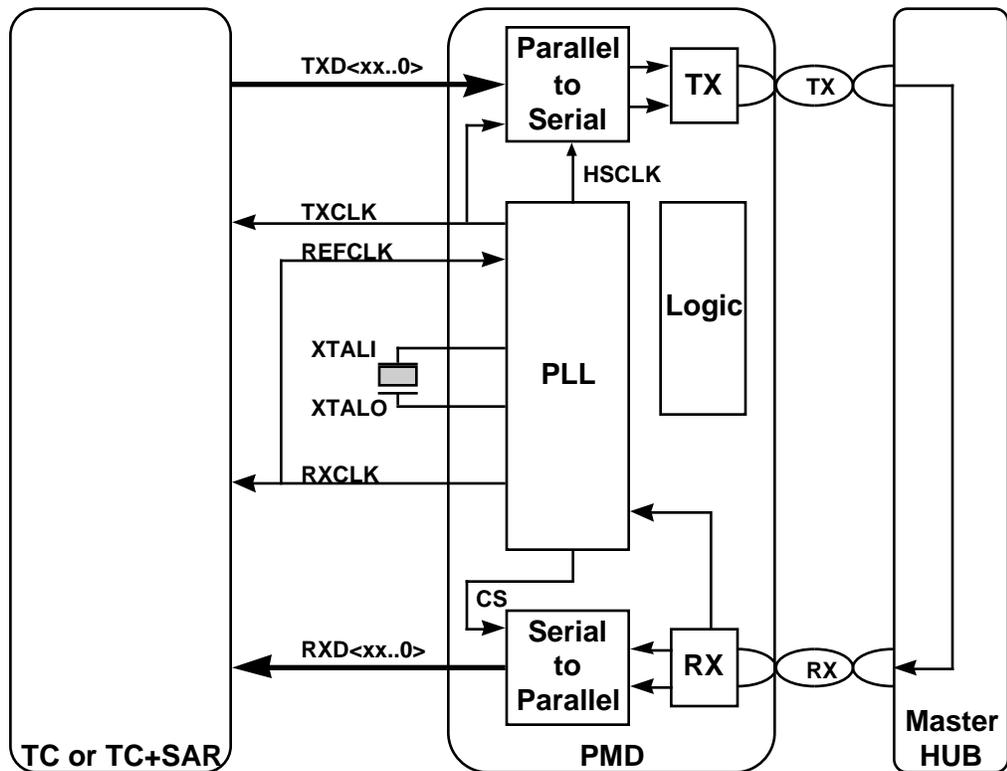
Figure 18: Parallel Interface Setup End Unit (Clock Slave)
