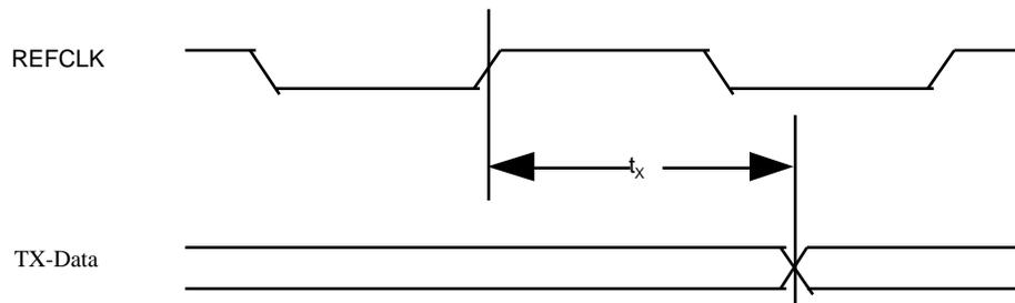
**Figure 1: Transmit Clock Referenced Timing**
