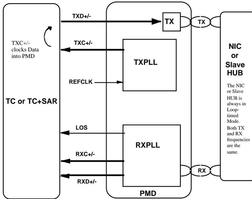
**Figure 15: Serial Interface Setup Network Unit (Clock Master)**
