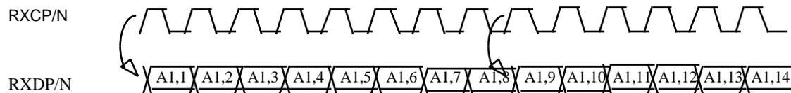
**Figure 5: Serial Receive Side Timing From PMD To TC**
