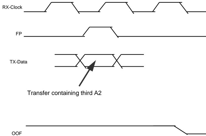
**Figure 3: Frame Detect Timing**
