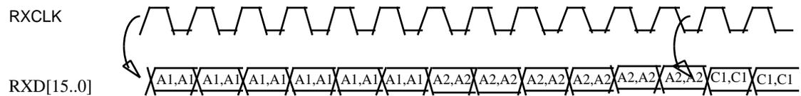
**Figure 9: 16 Bit Receive Side Timing From PMD To TC**
