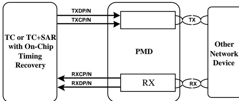
**Figure 14: Serial Interface Setup for PMD without Timing Recovery**
