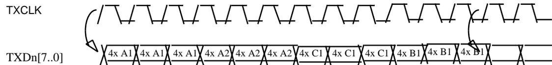
**Figure 10: Quad 8 Bit Transmit Side Timing From TC To PMD**
