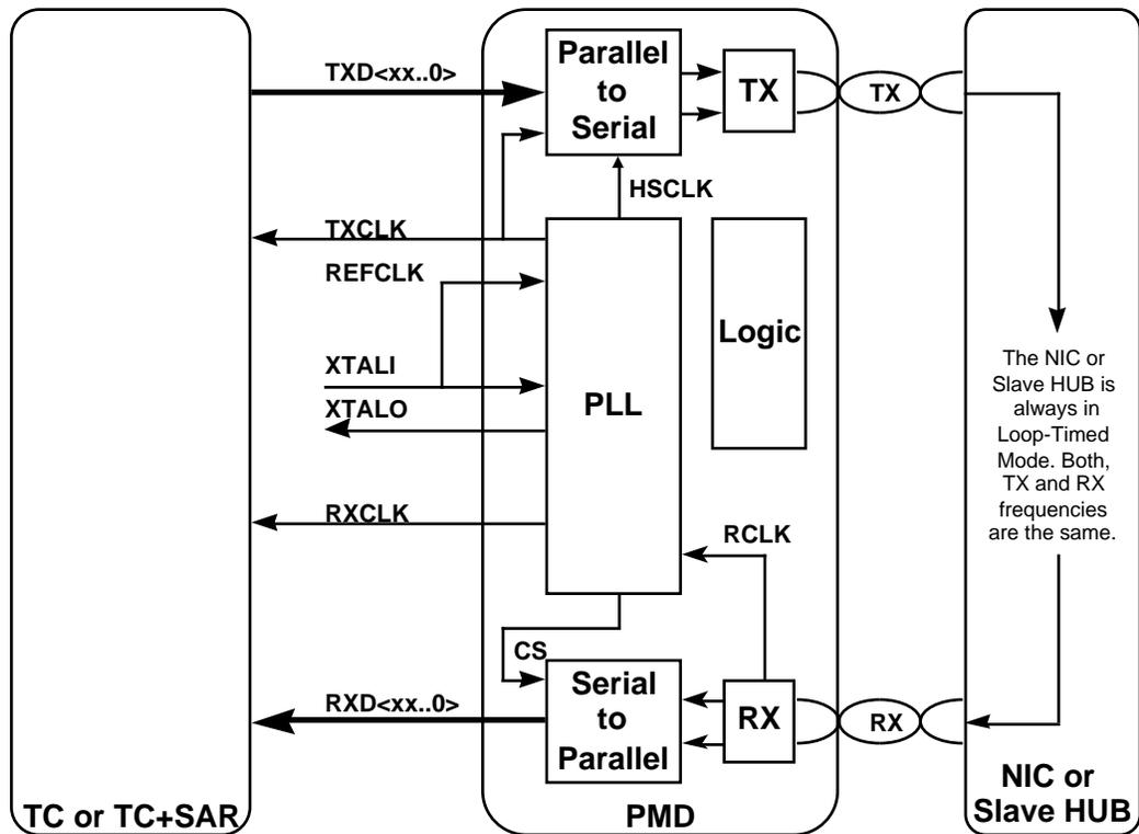
Figure 17: Parallel Interface Setup Network Unit (Clock Master)
