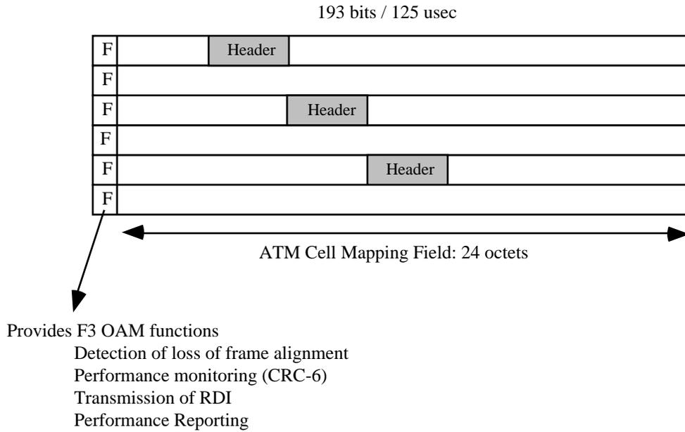
**Figure 4-1 ATM Cell Mapping**
