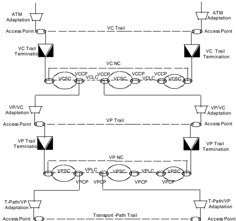
**Figure 4 Example of Layer Networks in ATM Context**
