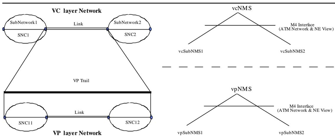
**Figure 6.5.1.1: Interlayer Trail Set-Up in a single Management Domain**
