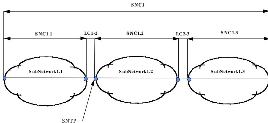
**Figure 6.3.2.2-a: Network Transport Architecture**
