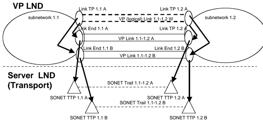
**Figure 4-3** Single VP Link / Multiple Server Trails
