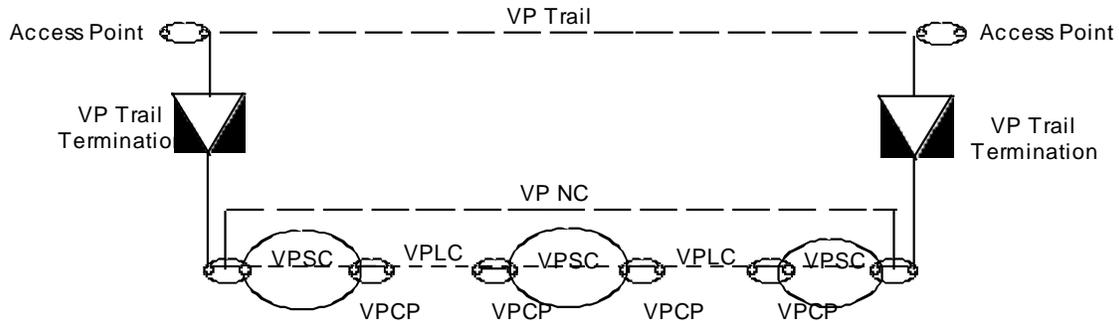
**Figure 2 ATM VP Layer Network**
