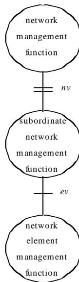
**Figure 3-1: M4 Network-View Logical Architecture**
