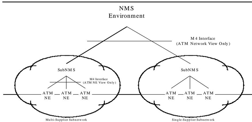
**Figure 3-2-1: Example of Network-View Management Physical Configuration**
