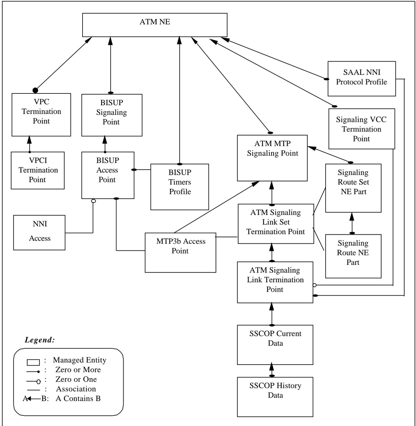
**Figure 3-6 Managed Entity Relationship Diagram - NNI Signaling (6 of 9)**
