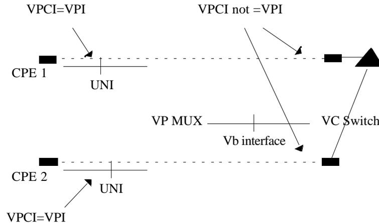
**Figure 2-11 Example: Signaling Configuration of Two Virtual UNIs**
