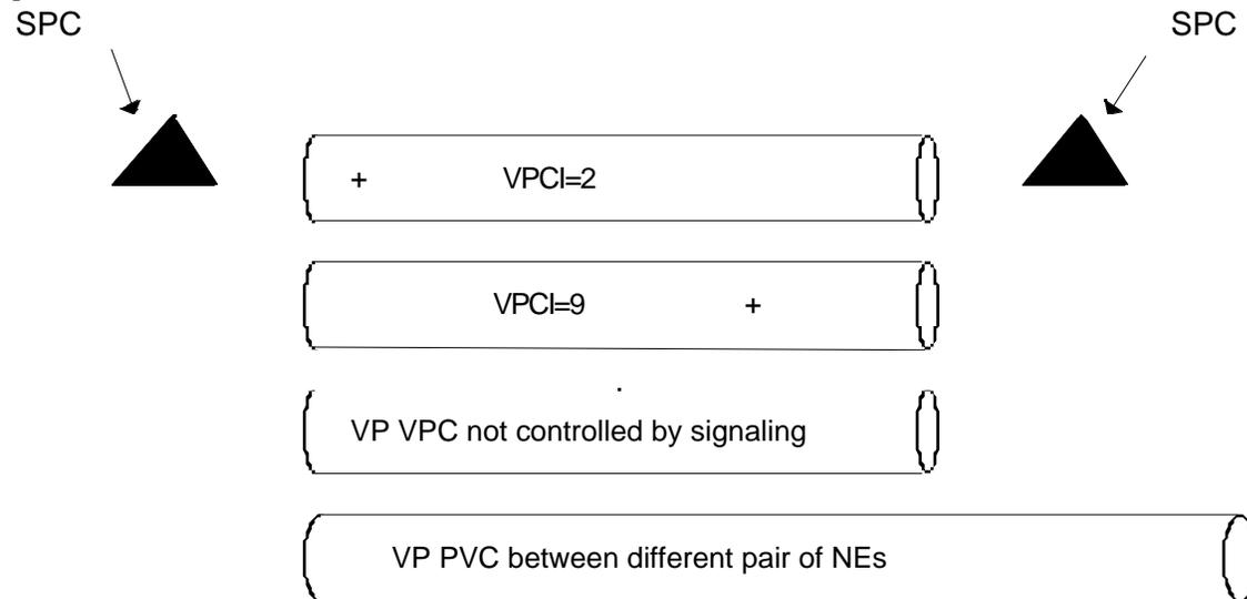
**Figure 2-12 Example: VPCI Configuration**
