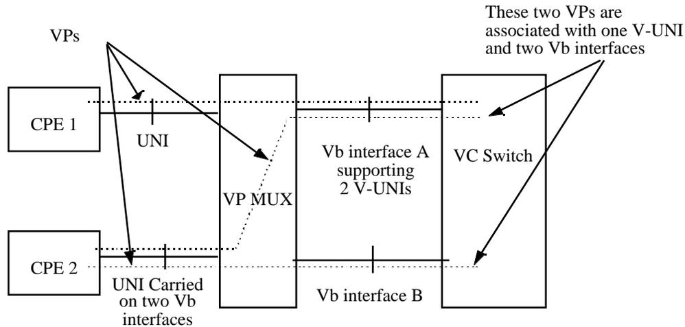
**Figure 2-3 Example: Configuration of Two Virtual UNIs on Two Multiple Vb Interfaces**
