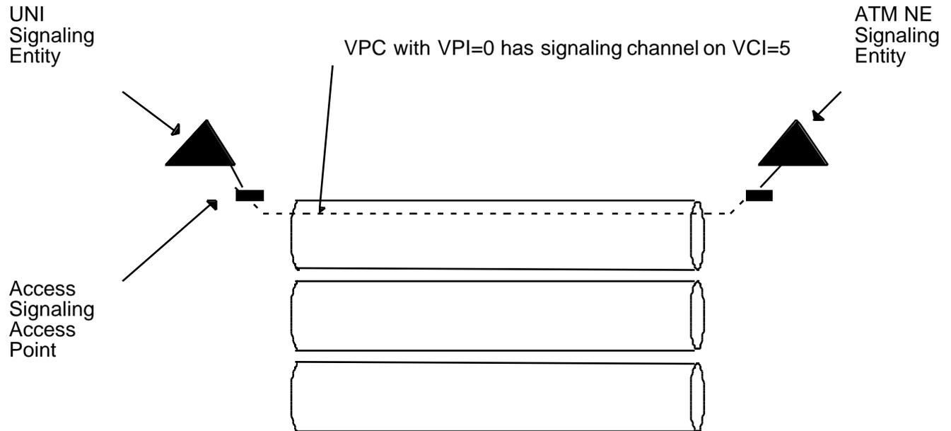
**Figure 2-9 Example: Interoffice Signaling Configuration**
