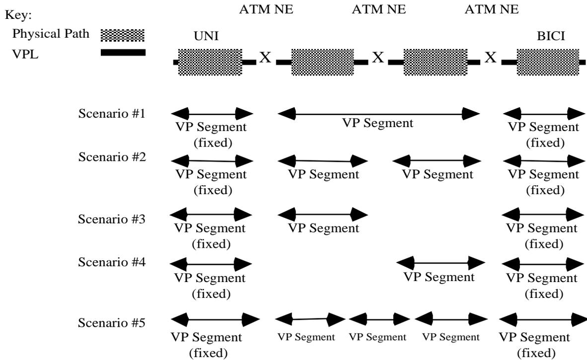
**Figure 2-6 Example VPC Segment Configuration Scenarios**
