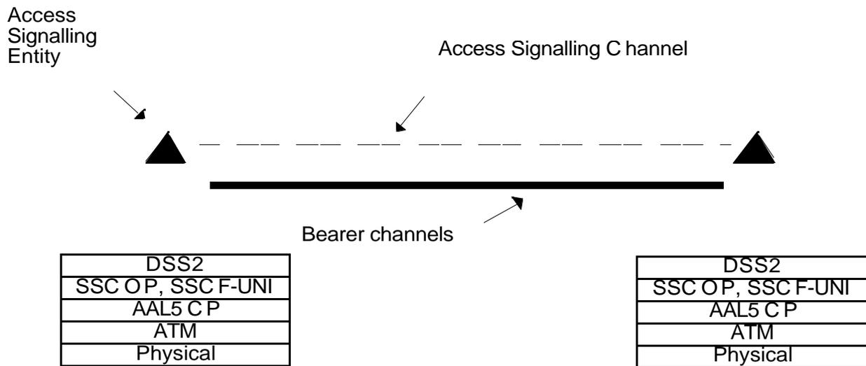
**Figure 2-7 Access Signaling**
