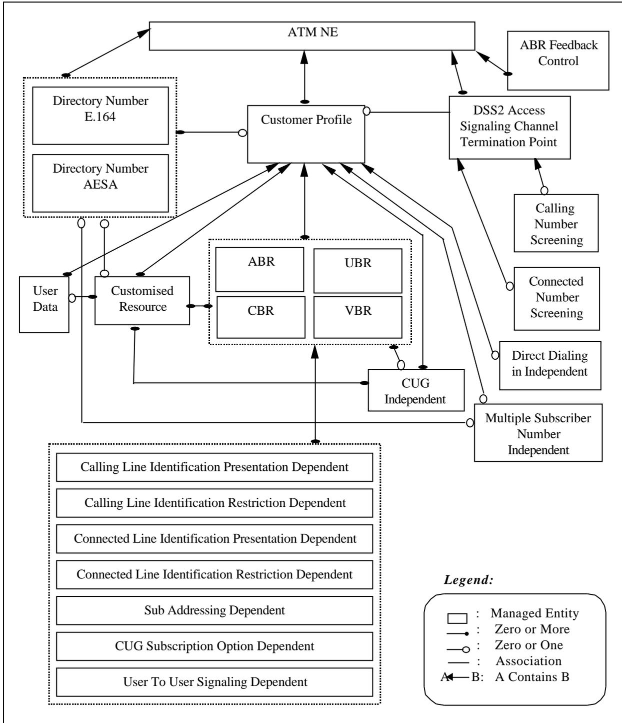
**Figure 3-8 Managed Entity Relationship Diagram – Call Routing Management (8 of 9)**
