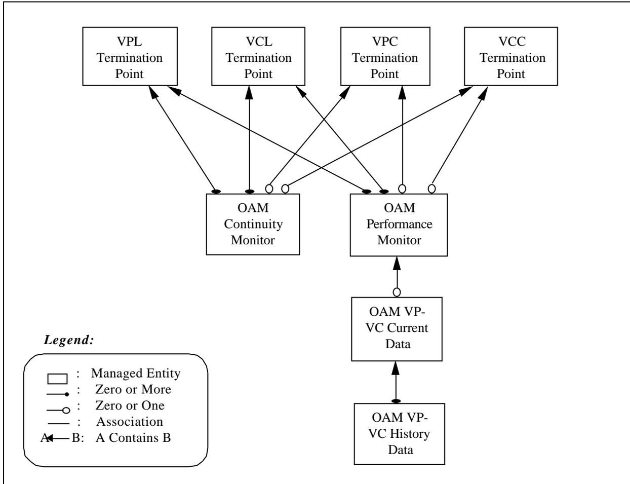
Figure 3-9 Managed Entity Relationship Diagram – OAM Flow Management (9 of 9)
