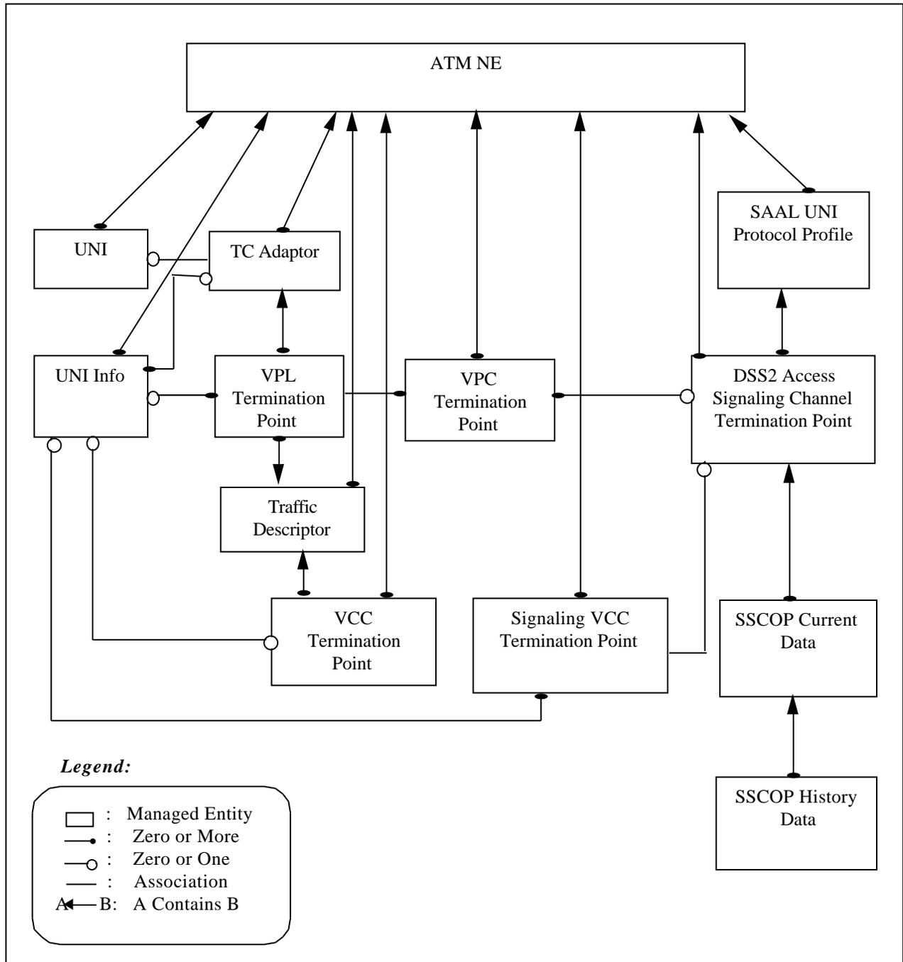
Figure 3-5 Managed Entity Relationship Diagram - Access Signaling (5 of 9)
