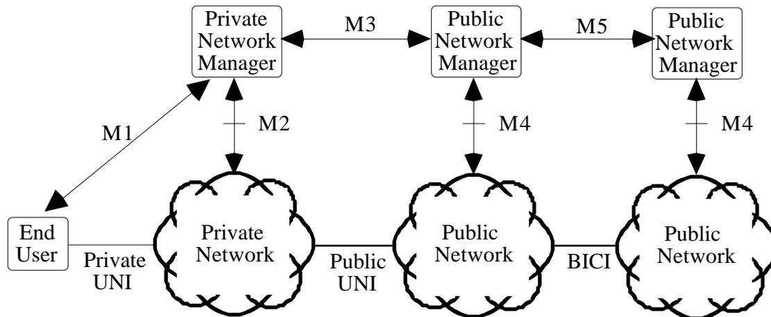
**Figure 1-1 The ATM Forum Management Interface Reference Architecture**
