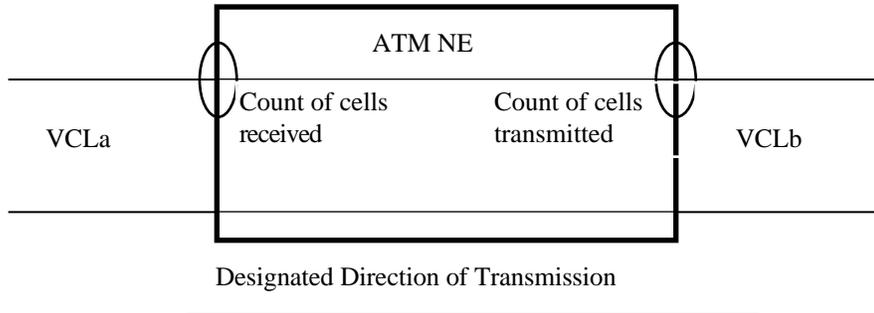
**Figure A-1** Estimation of CLR for a VCC
