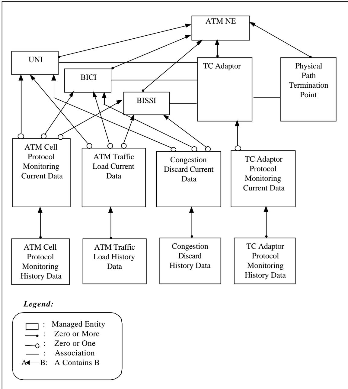
Figure 3-2 Managed Entity Relationship Diagram (2 of 9)
