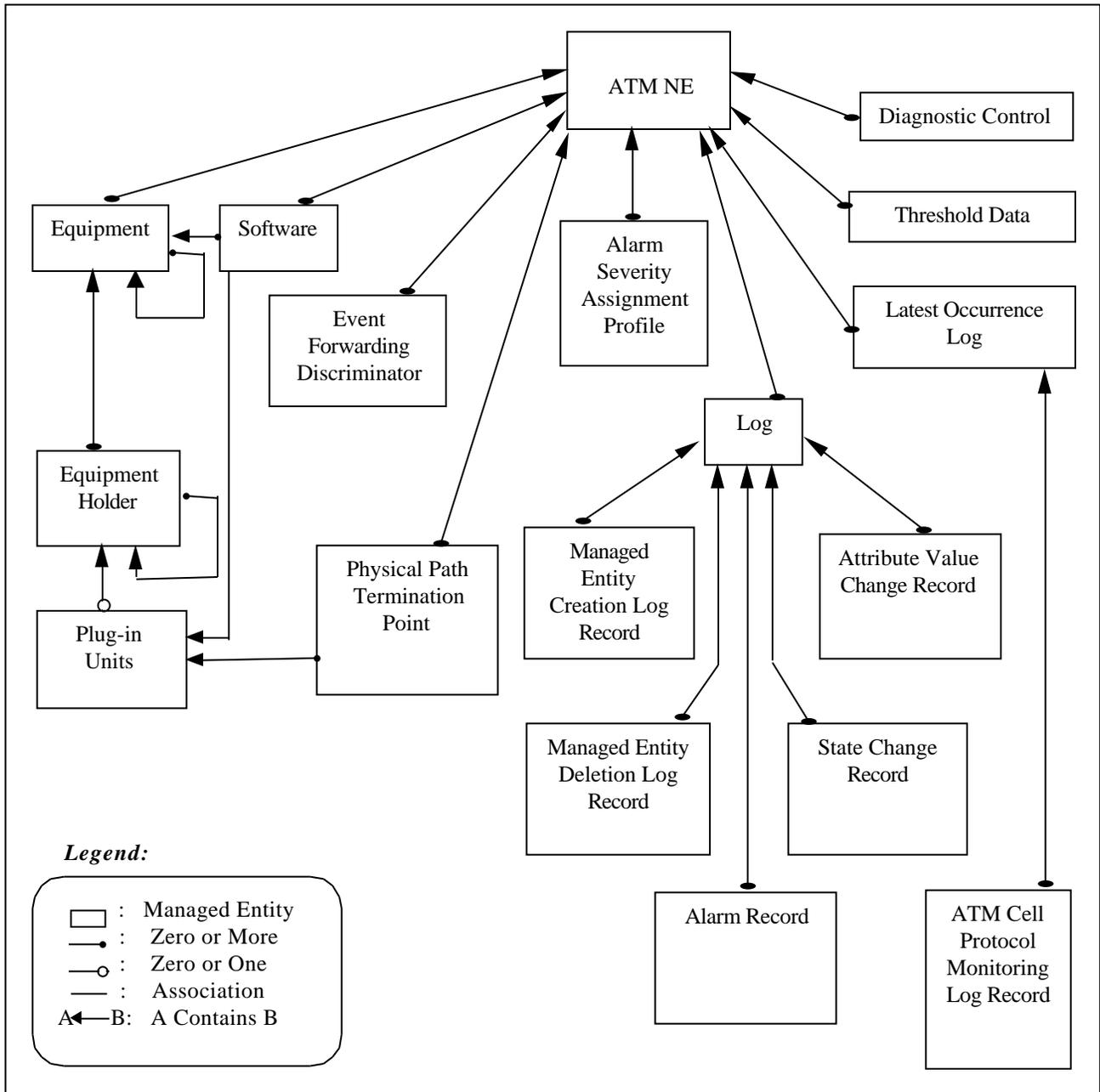
Figure 3-3 Managed Entity Relationship Diagram (3 of 9)
