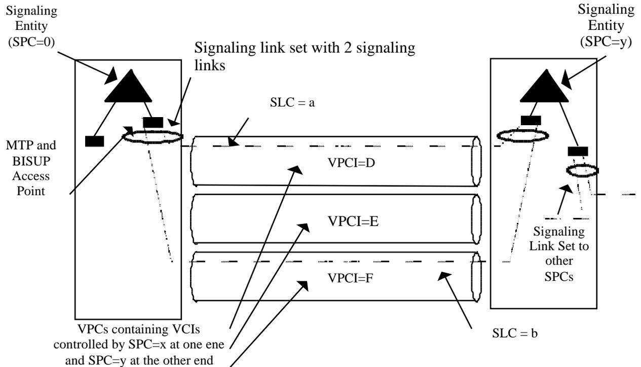
**Figure 2-10 Example: Interoffice Signaling Configuration**
