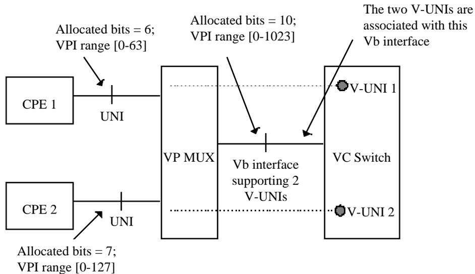
**Figure 2-2 Example: Configuration of Two Virtual UNIs**
