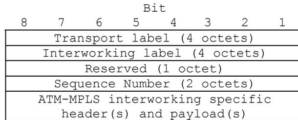
Note: bit 8 is the most significant bit
