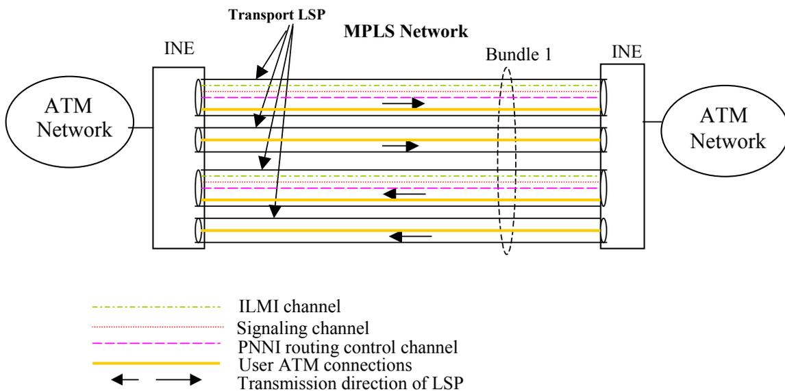
**Figure 7: Connections to Support Control Plane**
