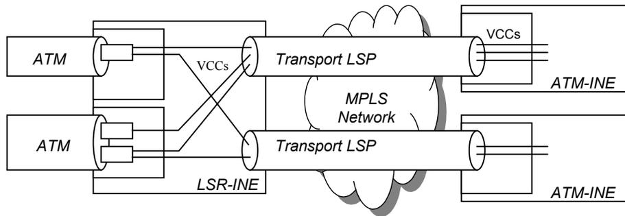
**Figure 13: Switching at Virtual Channel Level**
