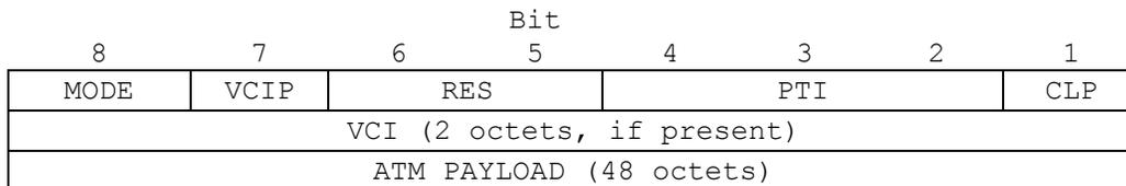
Note: bit 8 is the most significant bit
