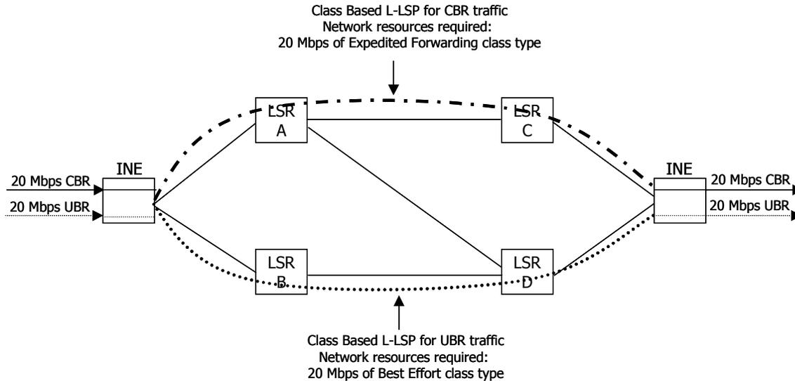
**Figure 19: Class Based L-LSP**
