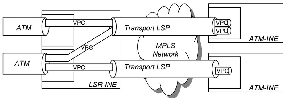
Figure 11: Switching at Virtual Path Level
