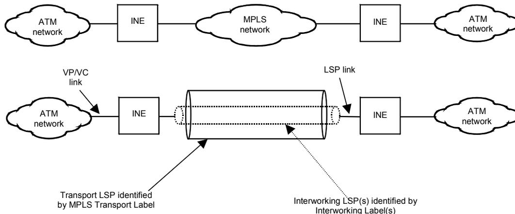
**Figure 3: Relationship between transport label and the interworking label**
