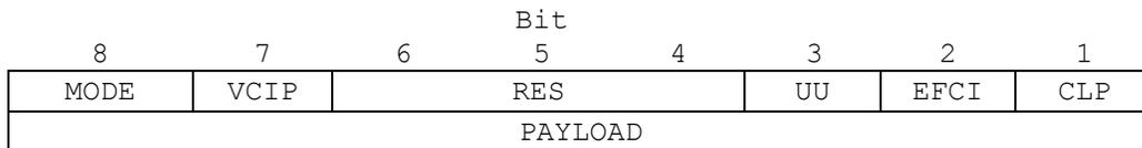
Note: bit 8 is the most significant bit
