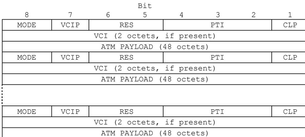
Note: bit 8 is the most significant bit
