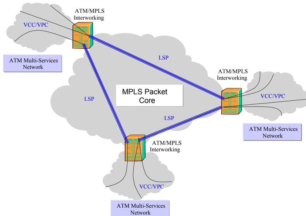
**Figure 8: Example of ATM-MPLS-ATM Network Interworking**
