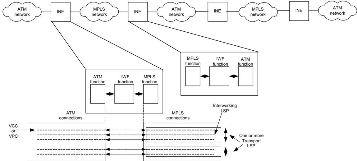
**Figure 15 INE High Level Functional Model**
