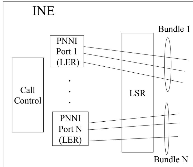
**Figure 9 Example Functional Model For an INE**
