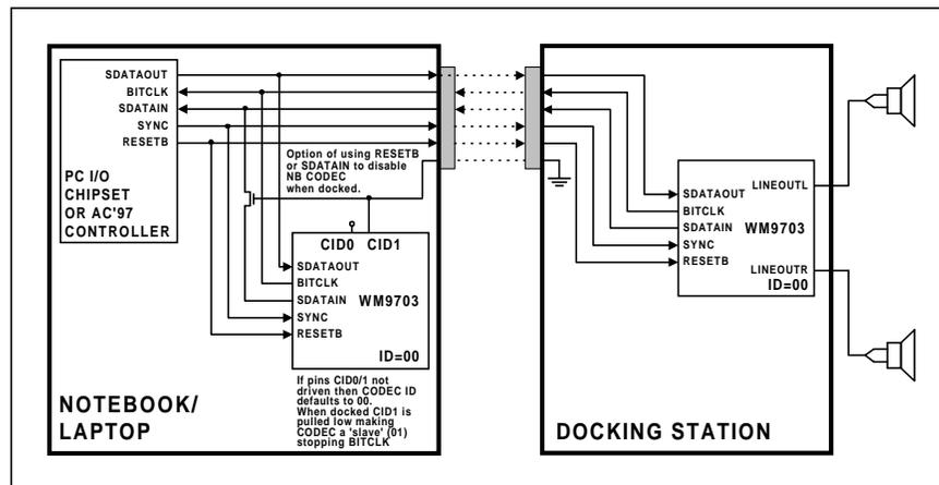
Figure 11 WM9703 in a Docking Station System
