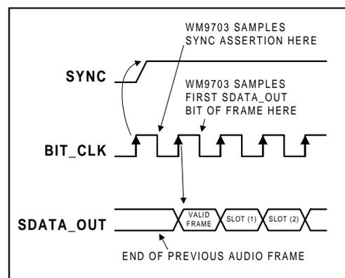
Figure 14 Start of an Audio Output Frame
