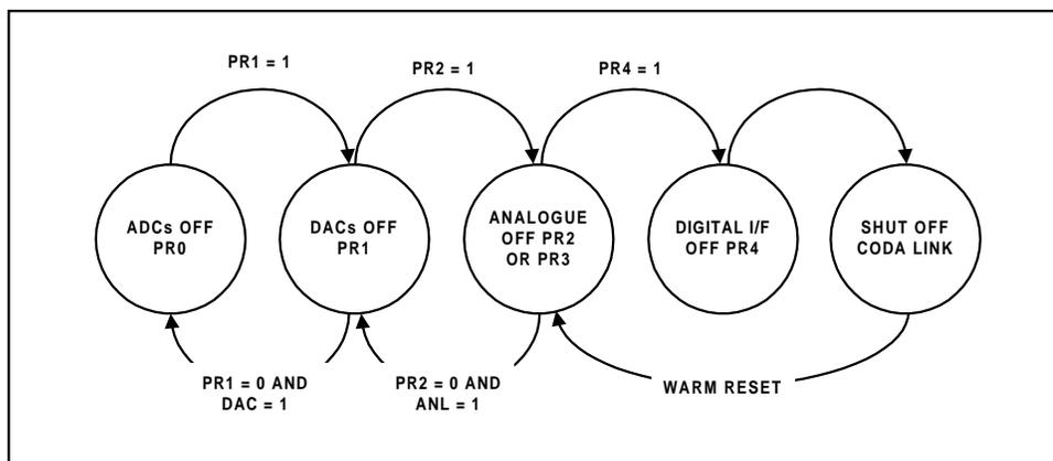
**Figure 18 The WM9703 Powerdown/Flow with Analogue Still Alive**
