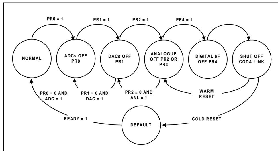
**Figure 17 An Example of the WM9703 Powerdown/Powerup Flow**
