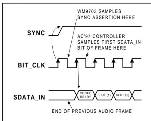
**Figure 16 Start of an Audio Input Frame**
