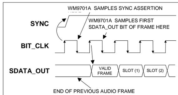
**Figure 9 Start of an Audio Output Frame**
