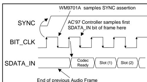
**Figure 11 Start of an Audio Input Frame**
