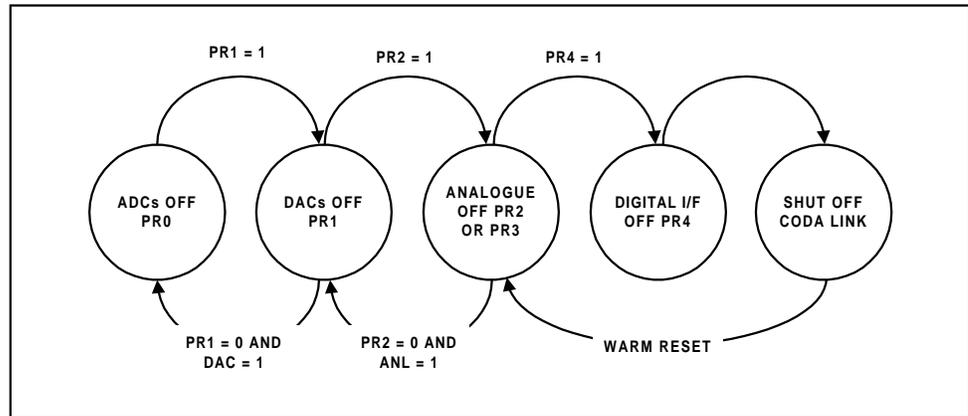
**Figure 13 WM9701A Power Down/Flow with Analogue Still Alive**
