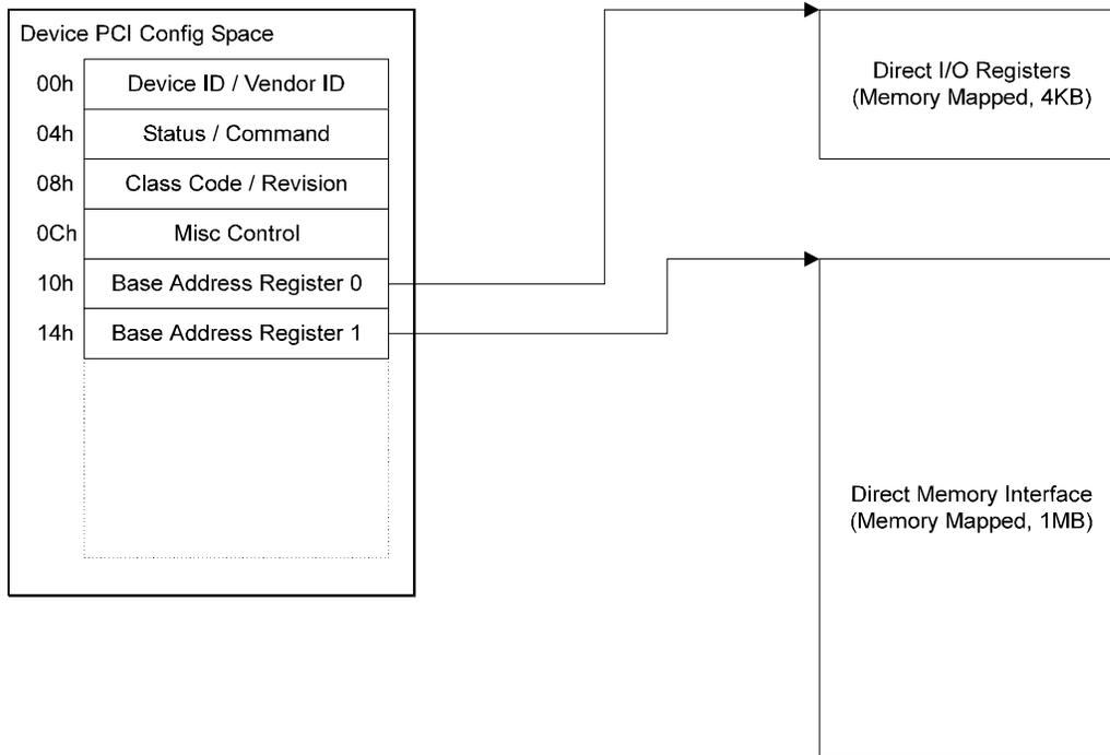
**Figure 11. CS4610/11 Host Interface Base Address Registers**
