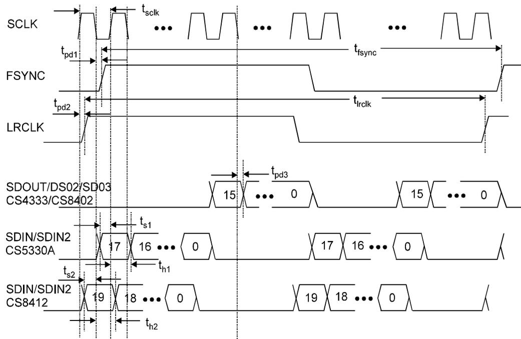
**Figure 5. Independent Timing Configuration**
