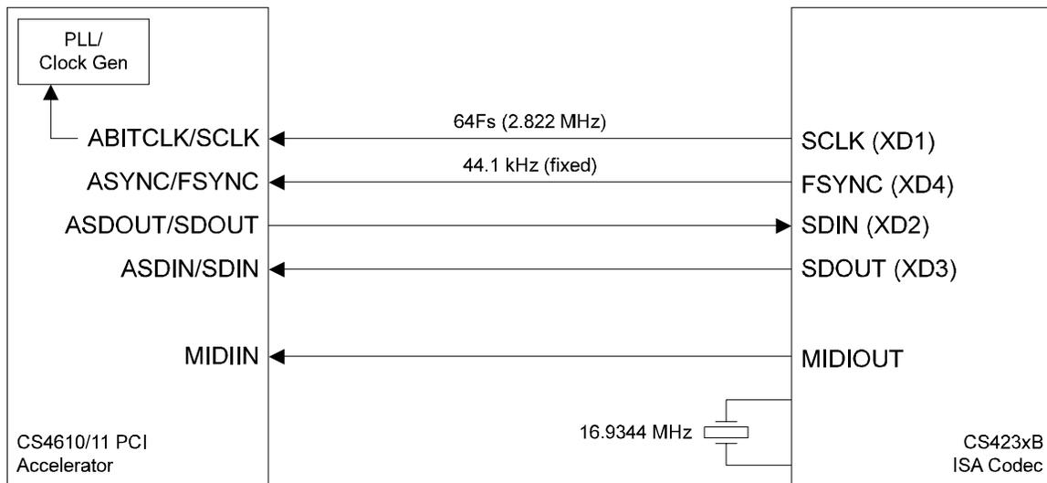
**Figure 12. CS4610/CS423xB Connection Diagram**
