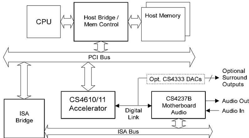
**Figure 9. CS4610/11 + CS423XB Motherboard Audio Configuration**
