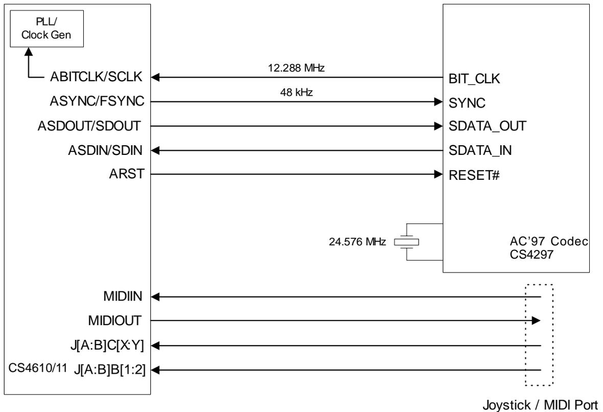
**Figure 16. CS4610/11 - AC '97 Codec Connection Diagram**
