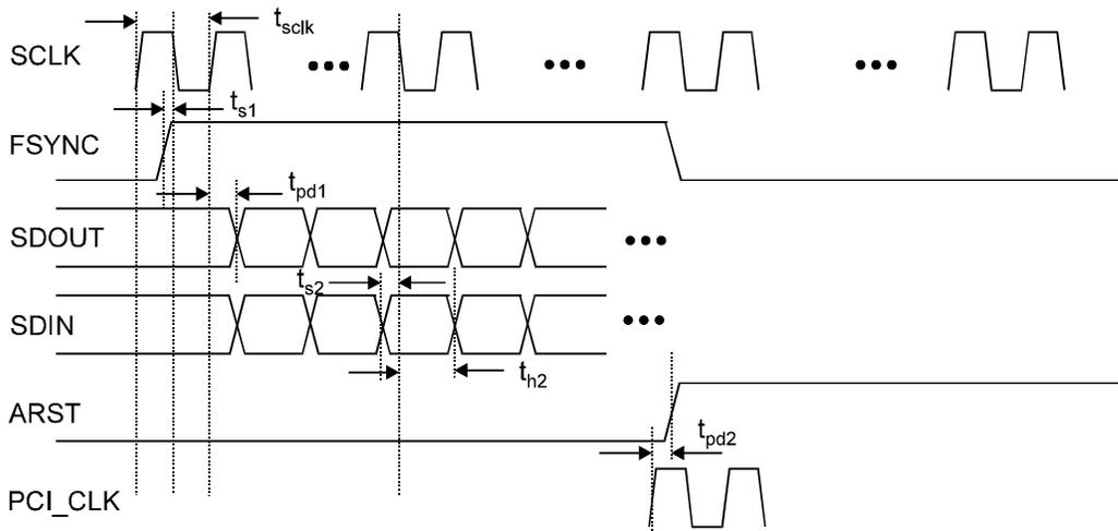
**Figure 4. AC97 Configuration Timing Diagram**
