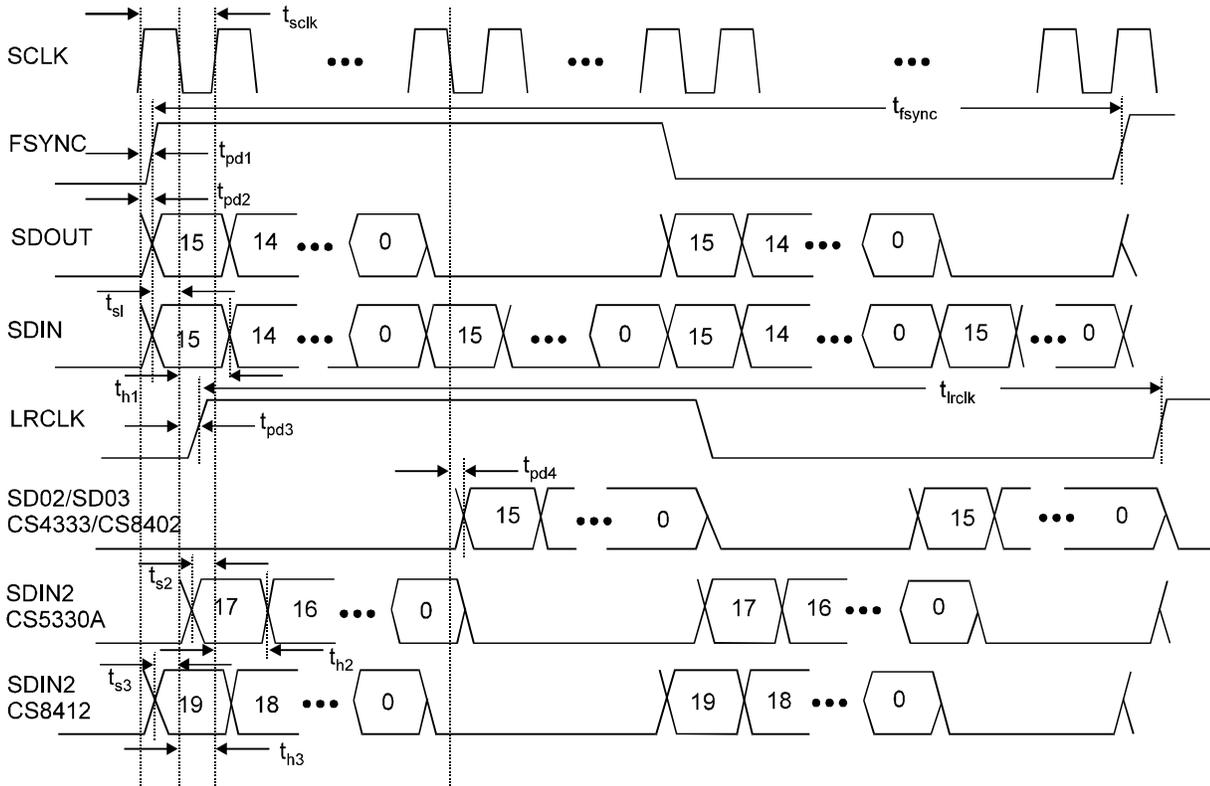
**Figure 3. CS4610/11 and CS423XB Link and AC3 Expanded Timing Diagram**
