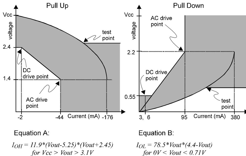
**Figure 1. AC Characteristics**
