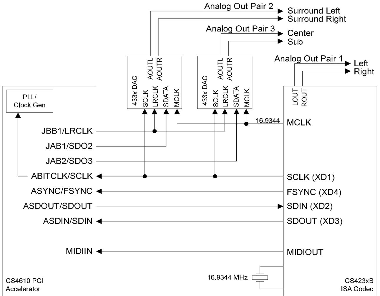
**Figure 14. CS4610 + CS423XB Expanded 6-Channel Output Configuration**
