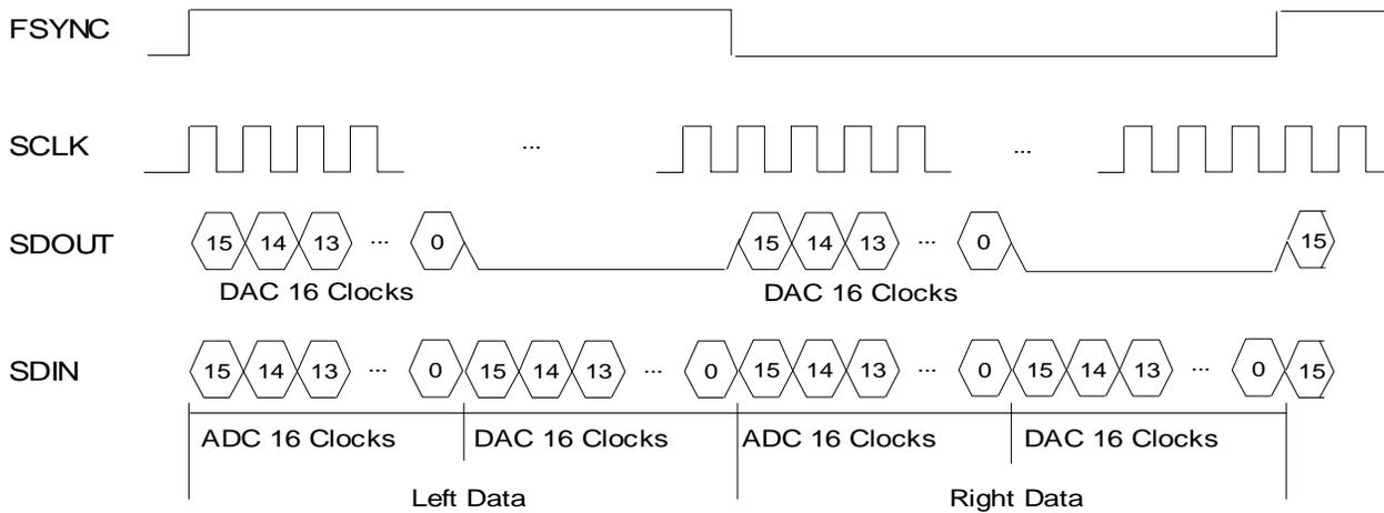
**Figure 13. Serial Audio Port Format for CS4610/11 + CS423XB Configuration**
