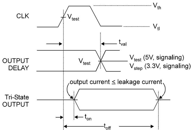
**Figure 8. Output Timing Measurement Conditions**
