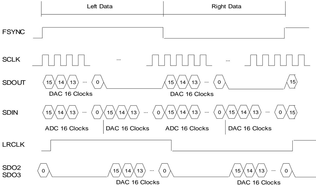
**Figure 15. Serial Audio Port Format for CS4610 + CS423XB Expanded Output Configuration.**
