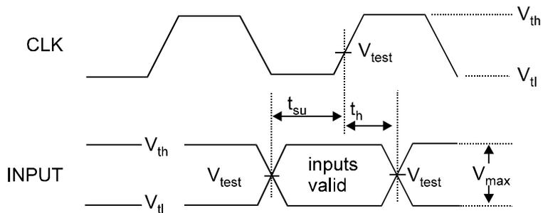
**Figure 7. Input Timing Measurement Conditions**
