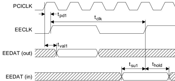
**Figure 6. EEPROM Timing Characteristics**
