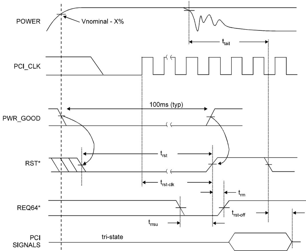
**Figure 2. Reset Timing**
