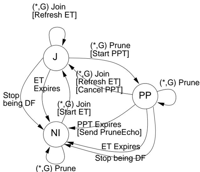
**Figure 1: Downstream group per-interface state-machine**
