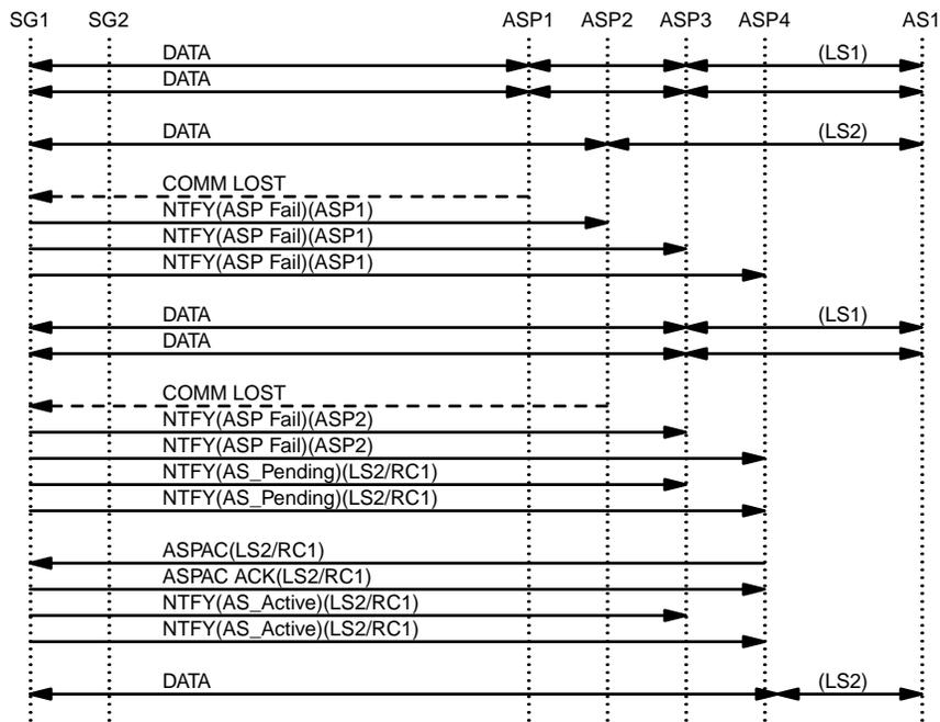
Figure 12. TUA Example – Failure of ASP1
