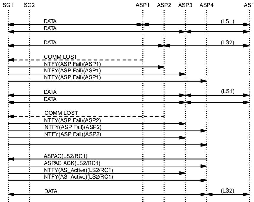
Figure 9. SUA Example – Failure of ASP1 and ASP2
