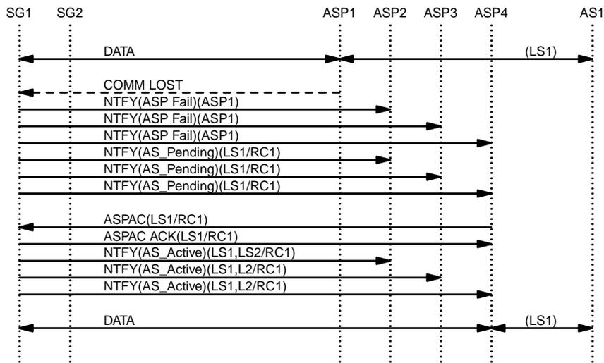
Figure 6. M3UA Example – Failure of ASP1
