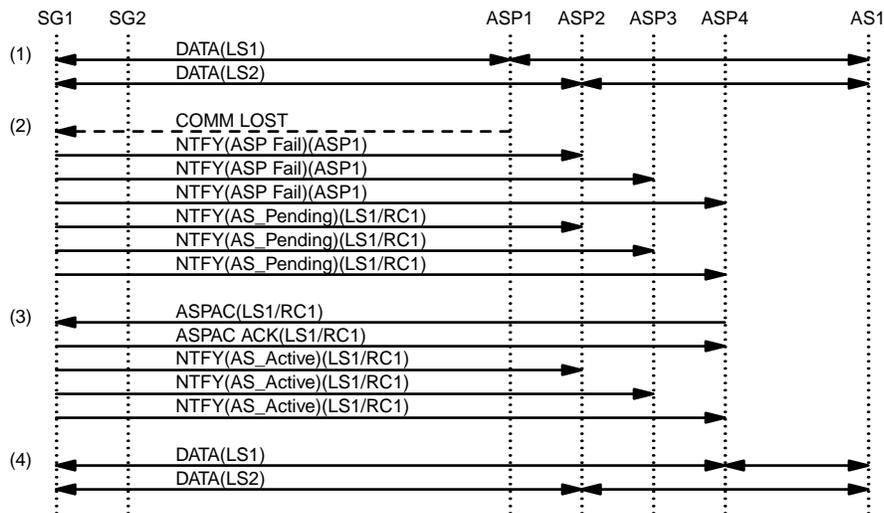
Figure 6. M3UA Example – Failure of ASP1
