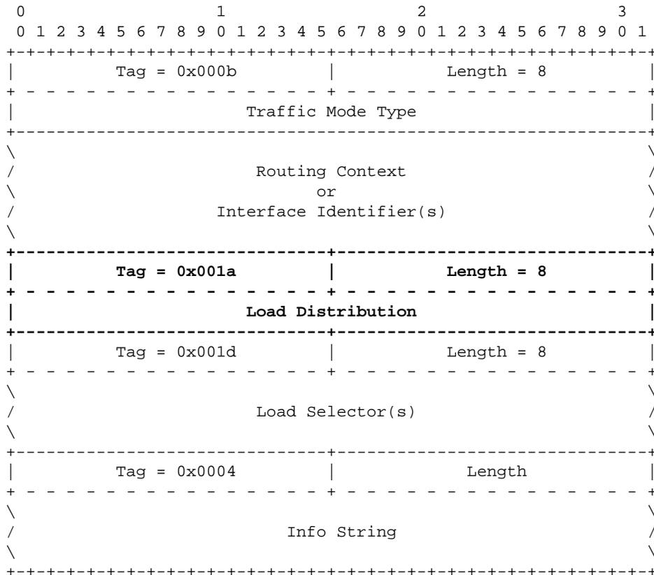
When an ASP has requested activation within a Load Group or the SG otherwise activates the ASP within a Load Group the SG responds with an ASPAC ACK message including the *Load Selector* that identifies the Load Group and optionally includes the *Load Distribution* for the Load Group in which the ASP has been activated. If the ASP included the *Load Distribution* parameter in the ASPAC message, the SG **MUST** include the *Load Distribution* parameter in the response ASPAC ACK message.
