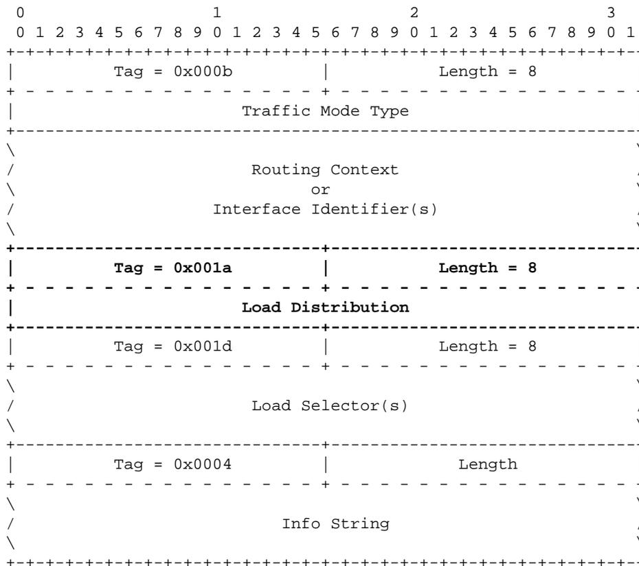
When an ASP wishes to activate only within a Load Group associated with an Application Server, it includes the *Load Selector* and *Load Distribution* parameters in the **ASPAC** message.
